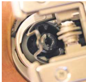
▲ The blade collar is set across the shaft when the blade isn't in place
